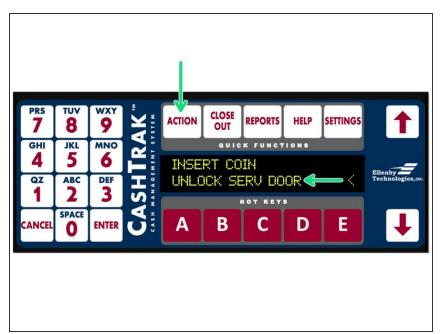
Open the service door by navigating to Action -->Unlock Serv Door
